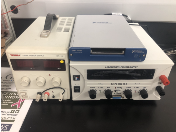
(a) EA-PS 3032-10 B power supply and NI USB-6341 DAQ
