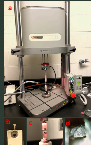
a) Instron E-1000 Electropulse fatigue testing system, b) Microsample , c) sample mounted in grippers, d) Fracture surfaces after fatigue test [13]
